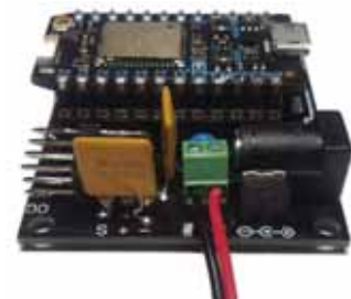
DC Power Supply Connected to +/-
